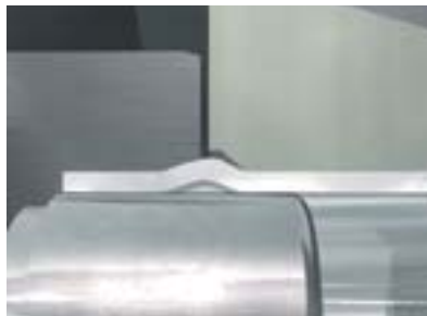
The tool shape defines the outer contour of the formed tube wall
