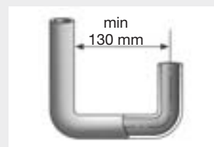
● Minimum clearance of U-shape bends
