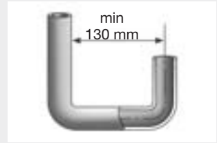
● Minimum clearance of U-shape bends
